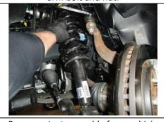
Remove strut assembly from vehicle
