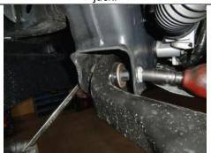
Loosen and remove front lower control arm bolt and nut
