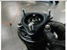
Install new strut extension with GOLD Flange Nuts, tighten.
