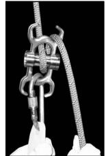
1) This is the beginning position for lowering or rappelling: Swing open the crossbar, reeve a bight of rope through the frame and around the crossbar. Bring the in feed line over a FORWARD Hyper-horn.
