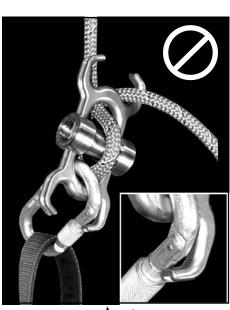
Make sure your carabiner is properly aligned and oriented before loading the SCARAB®, particularly on rappel. Small carabiners can sometimes jamb inside a Hyperhorn. This could possibly damage the carabiner or even lever the gate open. Pay attention to your system, before you weight it!
