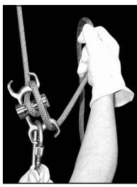
2) To add friction, wrap the in feed line around a rear horn (anchor or harness side) on the same side as you began with.
