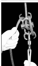
3) For rescue sized masses (200kg) cross to the empty forward Hyper-horn. For even more friction (for 280kg) wrap the remaining horn.
