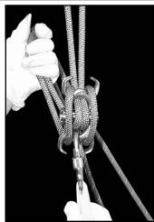
With small diameter ropes, such as this 8.1mm half rope, it is possible to rig two strands as if they were one strand of rope. Many configurations are possible depending on the diameter and construction of rope used.
