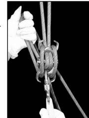
With small diameter ropes (not certified for NFPA G), such as this 8.1mm half rope, it is possible to rig two strands as if they were one strand of rope.
