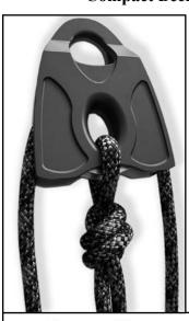
A very compact and efficient becket knot can be tied onto your Revolution Pulley as shown. The knot is historically known as an "Englishman's loop", but is more accurately named a "Blocked Slip Overhand". Using this knot in the Smart Becket allows more contraction of pulley systems in small spaces such as tripods.
