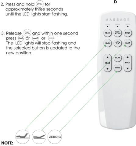
The three buttons shown above are pre-programmed with the manufacture's suggested bed position. No programming is necessary by the purchaser unless modified bed positions are desired.
