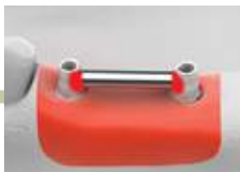
Connect the plastic bar in the middle of trimmed burn-out cylinders to help support the wax pattern. Wax pattern may have shrinkage.
