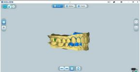
**9.2.4.** After scanning the buccal bite registrations, rotate the model and zoom the view to ensure that the bite is accurate and that there are no areas where the bite is mismatched. If necessary, you can delete the scanned occlusion and rescan.
