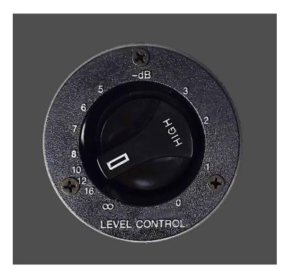
Note that the bezel is marked in minus dB, from minus infinity, namely off, to  $0\ dB$ , namely all the way up.
