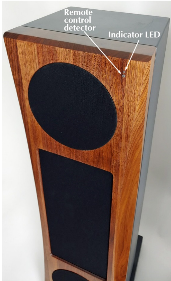
Indicator LED and IR sensor on a left master speaker.
