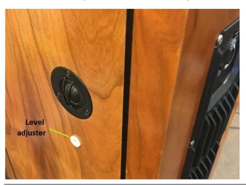
A small screwdriver is supplied for adjusting this control.
