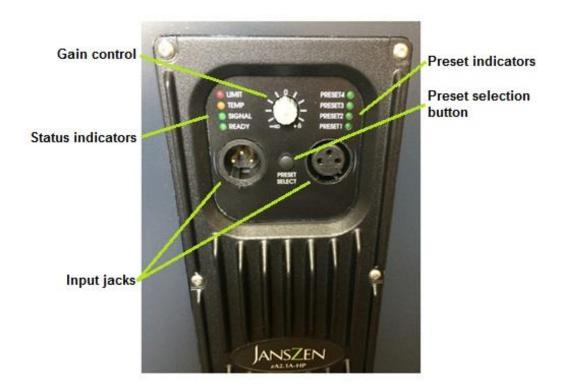
**Gain control**. Ideally, for the very best signal to noise ratio, the gain controls should be set so that the speakers are going about as loud as they can when your source level is set at maximum. Of course, there's always some uncertainty about what is "loud as they can," so rules of thumb are probably the best way to go, namely:
