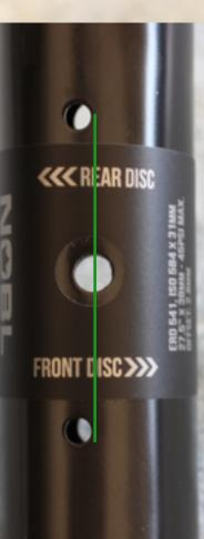
Valve Hole Decal Placement -Centred over the presto hole. Notice the orientation of the decal rear disc/front disc. compared to the centre line (green). Don't touch the back of the decal with your fingers, use decal backing. The area needs to be clean. Debris stuck to the back of the decal will show through the front once pressure is applied.
