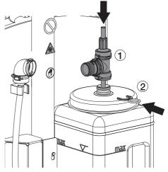
Connect the waste water connection to the rinsing hose.
