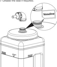
Light reduction and insertion of rinsing hose and waste water connection.
