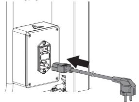
> Plug the mains plug into the power outlet.
