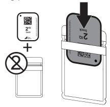
Pull off the adhesive strip, fold down the flap and close the light protection cover tightly by pressing together firmly.
