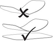
> Do not scratch the image plates. Do not subiect the image plates to pressure from hard or pointed objects.
