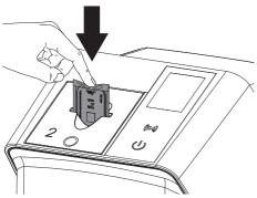
The light protection cover is held in place by the plate guide and is not drawn into the unit. Make sure that only the image plate, and not the light protection cover, is inserted into the unit. The image data is automatically transmitted to the imaging software.
