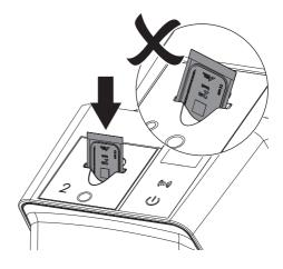
> Slide the image plate out of its light protection cover downwards into the device until the image plate is automatically drawn in.
