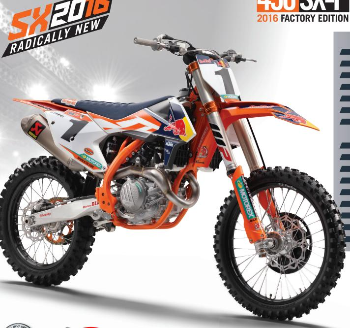
**ENGINE TYPE** Single cylinder, 4-stroke DISPLACEMENT 449.9 ccm BORE/STROKE 95/63.4 mm COMPRESSION RATIO 12.75:1 STARTER/BATTERY Electric starter / Lithium Ion12V 2.2 Ah FUEL SYSTEM Keihin EFI, throttle body 44 mm CONTROL 4 V / SOHC with rocker levers GEAR RATIOS 16:32 18:30 20:28 22:26 24:24- -FINAL DRIVE 13:48 COOLING Liquid cooling CLUTCH Wet multi-disc DDS-clutch, Brembo hydraulics IGNITION / ENGINE MANAGEMENT Keihin EMS
