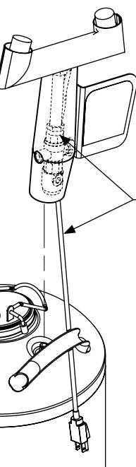
**A** Attach the eyewash yoke assembly to the tank. Max. torque 150 In-Lbs. Route the cable through the tank handle.
