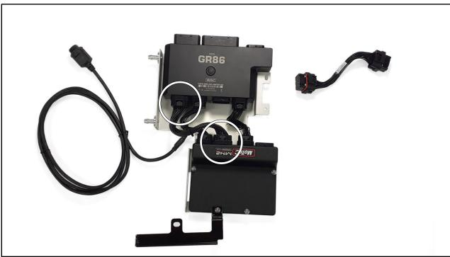
Step #13 Install Stub Loom C (#61475) in the location as shown above.
