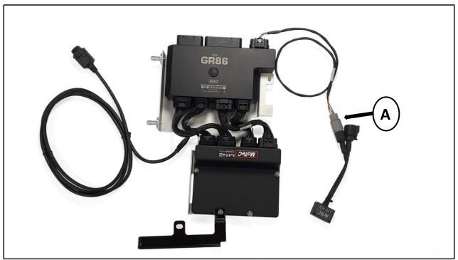
Step #16 Connect the LTC -LSU into the 4 pin DTM connector (A). Adaptor Kit Assembly is now complete.
