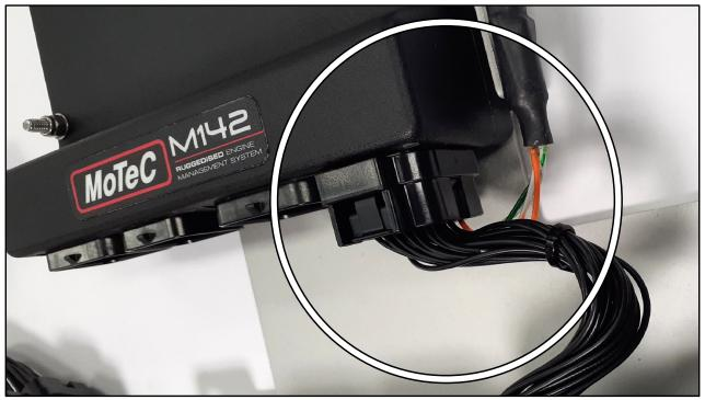
Step #12 When connecting stub loom D ensure the end with the ethernet cable is attached to the M1 side as shown above. This will provide communication with the M142 ECU when installed.
