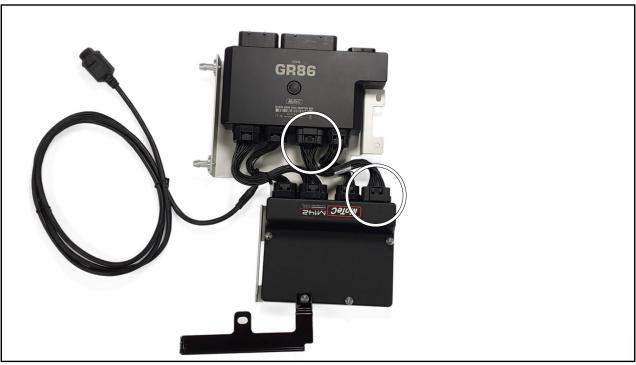
Step #14 Install Stub Loom A (#61254) in the remaining slot.
