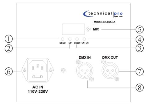
1. Menu Button: Press this button to switch between the multiple settings on the LG8xSEA. More details on the settings can be found below.
