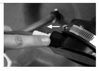
Push the longer hose over the exit connector (outward pointing arrow) of the pump.
