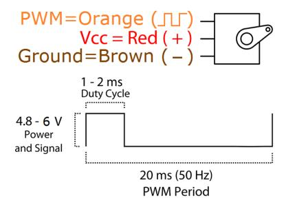
Position "0" (1.5 ms pulse) is middle, "90" ( $\sim$ 2 ms pulse) is all the way to the right, "-90" ( $\sim$ 1 ms pulse) is all the way to the left.
