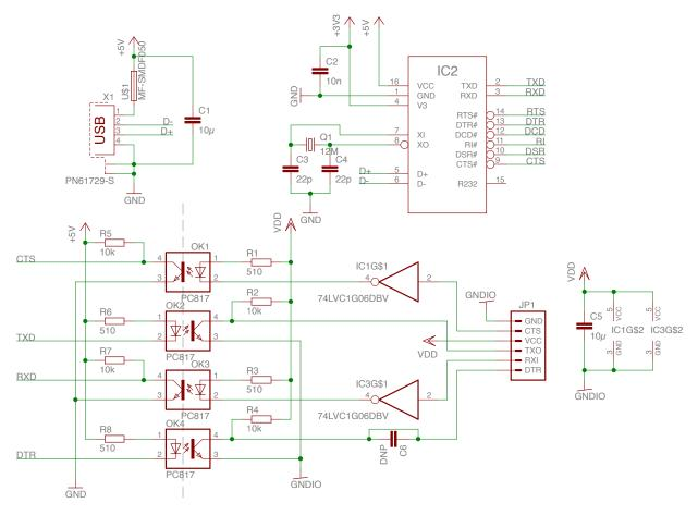
This adapter provides optically isolated inputs and outputs with 4 PC817 optoisolators. Respect the isolation border when laying out the board, and if possible, cut slots under the optoisolators. The two 74LVC1G06 is optional, but helpful when the input pins cannot source too many current.
