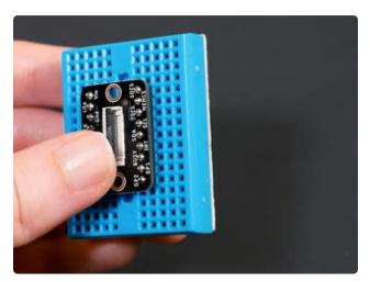
Then, insert the EYESPI cable into the open FPC connector by sliding the cable into the connector. You want to see the blue stripe facing up towards you. This inserts the cable pins into the FPC connector.
