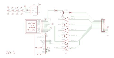
For the level shifter we use the CD74HC4050 which has a typical propagation delay of ~10ns
