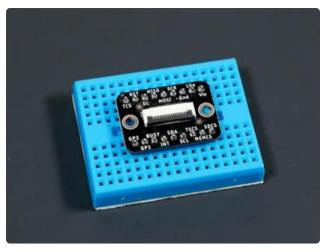
To begin inserting an EYESPI cable to an FPC connector, gently lift the FPC connector black latch up.
