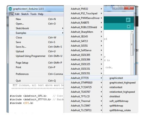
After restarting the Arduino software, you should see a new example folder called Ad afruit\_ST7735 and inside, an example called graphicstest.
