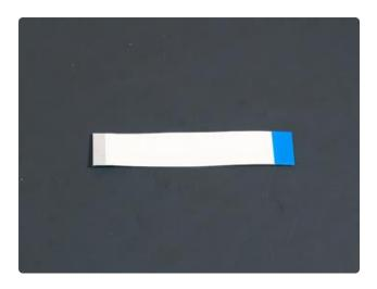
Each EYESPI cable has blue stripes on either end. On the other side of the cable, underneath the blue stripe, are the connector pins that make contact with the FPC connector pins on the display or breakout.
