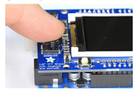
The 5-way joystick on the shield is great for implementing menu navigation or even for use as a tiny game controller. To minimize the number of pins required, the joystick uses a different resistor on each leg of the control to create a variable voltage divider that can be monitored with a single analog pin. Each movement of the joystick control connects a different resistor and results in a different voltage reading.
