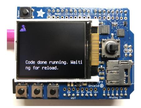
Finally, we place an infinite loop at the end and constantly read the buttons. If a button is detected as being pressed, a message specifies which one. Multiple buttons can be pressed at the same time. We also provide an optional small delay to allow you to adjust how quickly you want the buttons to read in case you want to debounce the output.
