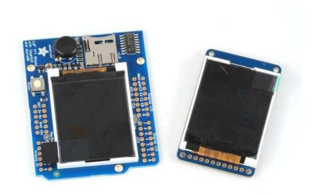
The 1.8" display has 128x160 color pixels. Unlike the low cost "Nokia 6110" and similar LCD displays, which are CSTN type and thus have poor color and slow refresh, this display is a true TFT! The TFT driver (ST7735R) can display full 18-bit color (262,144 shades!). And the LCD will always come with the same driver chip so there's no worries that your code will not work from one to the other.
