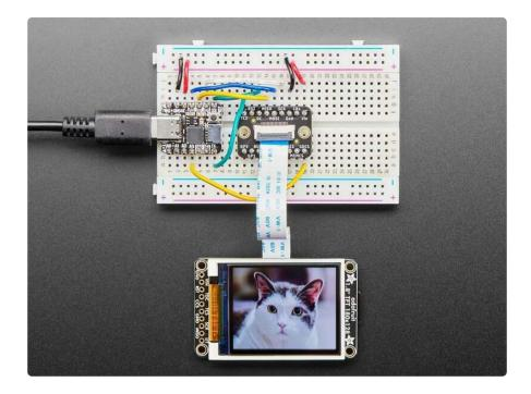
This display now comes with an EYESPI connector. This connector allows you to connect your display without soldering. There are <a href="EYESPI cables">EYESPI cables</a> () available in multiple lengths, which means you can find one to fit any project. This is especially useful if your project requires the display to be freestanding, and not tied directly into a breadboard. Inspired by the popularity of STEMMA QT, it provides plug-n-play for displays!
