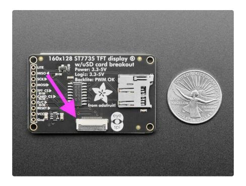
The EYESPI cables are 18 pin 0.5mm pitch flex cables. They are  $^{\sim}$ 9.6mm wide, and designed to fit perfectly into the EYESPI connector. Adafruit currently offers EYESPI cables in three different lengths: 50mm (), 100mm (), and 200mm ().
