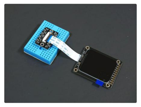
You can connect an EYESPI compatible display to the EYESPI breakout board using an EYESPI cable. An EYESPI cable is an 18 pin flexible PCB (FPC). The FPC can only be connected properly in one orientation, so be sure to follow the steps below to ensure that your display and breakout are plugged in properly.
