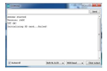
The sketch waits until the serial port is opened (you can make it auto-start once you know things are working by removing the while (!Serial); line
