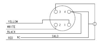
FIGURE 15. XLR Connector Wiring, 750 Model -219
