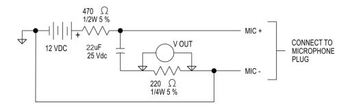
FIGURE 1. Airman 750 Headset Boom Microphone Sensitivity Check Test Circuit
