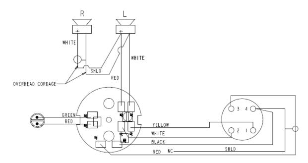
FIGURE 6. Airman 750 Headset Model 219 -Wiring Diagram
