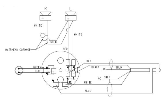
FIGURE 5. Airman 750 Headset Model -218 Wiring Diagram
