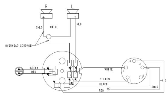
FIGURE 2. Airman 750 Headset Model -210 Wiring Diagram
