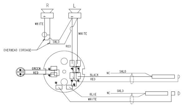
FIGURE 1. Airman 750 Headset Model -200, -220, -300 Wiring Diagram
