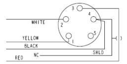
**FIGURE 11.** XLR Connector Wiring, 750 Model -205, -208, -210
