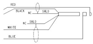
FIGURE 13. PJ-068 Connector Wiring, 750 Model -218
