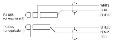
FIGURE 17. PJ055 and PJ068 Connector Wiring, 750 Model -220
