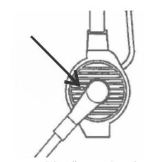
FIGURE 2. Gain Adjustment Control
