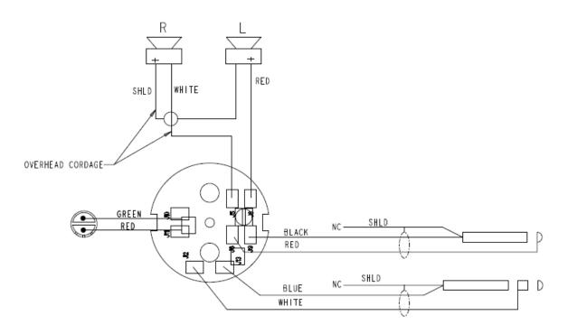
FIGURE 4. Airman 750 Headset Model -212 Wiring Diagram
