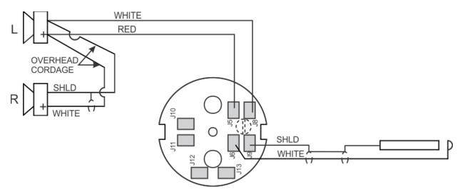
FIGURE 7. Airman 760 Headphone Model -200 Wiring Diagram
