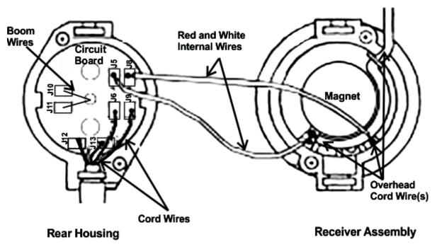
FIGURE 2. Circuit Board/Receiver/Cord Wiring
