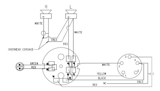
FIGURE 3. Airman 750 Headset Models -205, -208 Wiring Diagram
