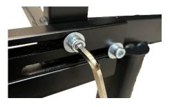
through the bracket. Ensure the bracket is in the correct position by lowering the backrest to the flat position and aligning the bracket approximately 5mm away from the backrest edge. Tighten the bolts into the bed frame using the Allen key. Repeat for the opposite side.
