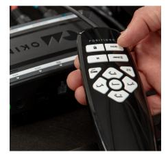
If your motion base does not pair first time or becomes disconnected, there is a PAIR button on the control box. Press this to reactivate pairing mode and the control box light will illuminate blue to indicate the base is ready to pair.
