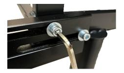
through the bracket. Ensure the bracket is in the correct position by lowering the backrest to the flat position and aligning the bracket approximately 5mm away from the backrest edge. Tighten the bolts into the bed frame using the Allen key. Repeat for the opposite side.
