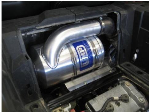
Pic 5-Canister installed with room for 45 elbow and inlet hose.
