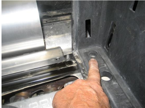
Pic 3-Right side front bed bolt and 17/64" hole for bracket to left
