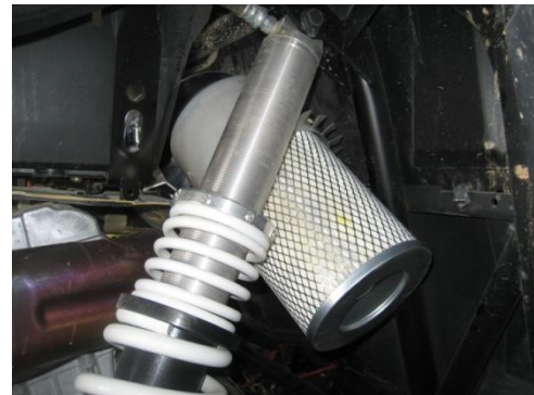
Pic 6- Tight squeeze of element servicing.
