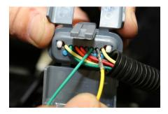
5. Close Cover – Run our adapter cord along side the OEM harness and snap shut, re-install plastic locking cover
