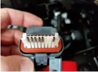
3. Remove Plugs – Using a pair of needle nose pliers remove the plugs from wire port 6 and 7.
