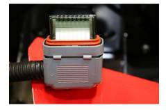
2. **Remove Connector Lock** – Using a small screw driver push in on both sides of the at the white connector shown below and slide lock off
