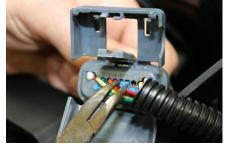
4. **Insert Wires** – Insert the Green Wire into the port 6, plug the yellow wire into port 7.
