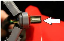
6. **Unplug** – the front harness from the TSS and insert the adapter in between the two connectors.
