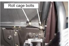
2. Install hinge bracket using the stock upper sidebar bolt
