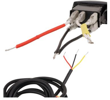
**Note** | Wires for Spectrum switch/wiring harness Yellow wire (+12v) = Constant power Black wire = Ground Red wire = Trigger (or switch) power
