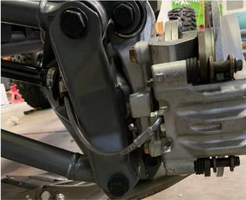
26. Remove the brake caliper from the brake rotor using the 15mm box end wrench.
