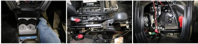
2. Using the provided Self Tapping Screw mount the Control Module on the frame in the dash.
