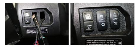
**Dielectric Grease** - Just like the OEM uses on their switches, we recommend using Dielectric Grease on all switch terminals, this keeps the water out, thereby reducing corrosion and helps increase reliability! Open the grease and put on the switch terminals and the connector terminals on both the Turn and Horn switches, the more the better.
