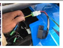
The SELF-CANCELING FLASHER RELAY has a timing circuit that will cancel the turn signals after three minutes and thirty three seconds. The timer is reset whenever the turn signal switch is returned to the center/off position.
