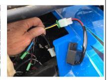
NOTE: Do NOT connect the front or rear turn signal harness to the TURN SIGNAL/HORN SWITCH at this time.
