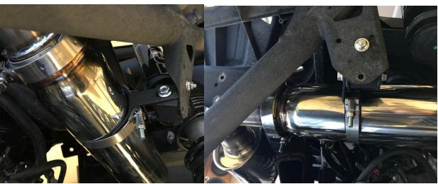
Step 6: Install rear exhaust mount to the left side of the factory muffler mounting point. Install smaller exhaust bracket to the rear exhaust mount. Leave bolts just lose enough to be able to adjust mount and bracket.
