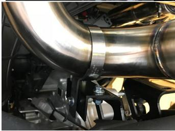
Step 8: Adjust exhaust and mounts to center exhaust tip to the center of the X3. Also use the the rear plastic to check for centering the exhaust. Once exhaust is positioned to your liking go through and tighten all the bolts, nuts, and clamps. When finished tightening everything double check fitment and re-adjust if needed.
