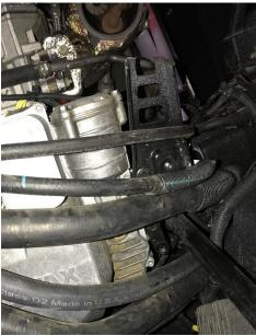
Step 3: Replace exhaust/hose support bracket with new hose support bracket
