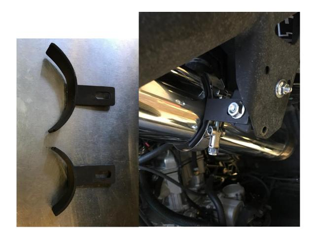
Step 5: Install forward exhaust section to turbo using new V-band clamp. Use 4-inch T-bolt clamp to clamp the exhaust to mounting bracket. Snug up the V-band and T-bolt to be able to hold a position but still be able to be move in to need positions.
