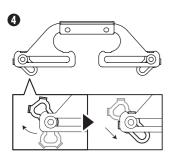
Set the locking units and adjust them as shown above. Confirm that all four locking units on both handles are locked.
