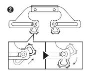
Unlock the four locking units and adjust the handles as shown above. If the locking units are not firmly facing downwards, the pieces will interfere with one another when the box is opened or closed.
