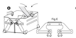
Hold both sides of the box, and close it until the sliding pins are as shown in Fig. E.
