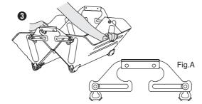
Hold both sides of the box and open it until the sliding pins are as shown in Fig. A.
