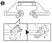
Set the locking units and adjust them as shown above. Confirm that all four locking units on both handles are I ocked.
