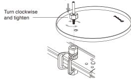
③After tightening the fixing shaft screw completely, align the tray to the desired position. Once aligned, screw the fixing nut clockwise until the tray stops moving, then tighten.
