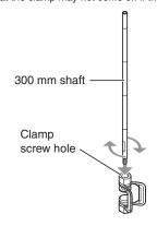
②Tighten the other CK-300 clamp to the point where it can be moved to the left and right, and temporarily fix it to the table.
