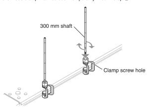
④Insert U-shaped bracket joint bolt into the screw hole of the 300 mm shaft, rotate it clockwise, and tighten both sides in order. If the screw holes of the joint bolts do not match, adjust the position of the CK-300 clamp that was temporarily fixed in step ② to the left or to the right, and tightly screw it in both the left and right joints of the U-shaped bracket until there is no looseness.
