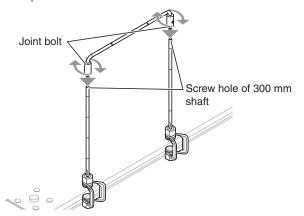
(5) In the same way, attach the U-shaped bracket joint to the screw hole at the bottom of the clamps until there is no looseness and so that it does not wobble.
