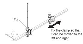
③Turn the 300 mm shaft clockwise to tighten in the same way as in step ①, and fix it to the CK-300 clamp that has been temporarily fixed in step ②.
