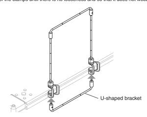
⑥Tighten the clamp that has been temporarily fixed until there is no looseness. Finally, check it again for any looseness.
