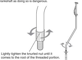
3 After tightening the threaded portion of the crank shaft all the way, turn the crank shaft in the opposite direction to set it to the desired position of the lantern hanger. After finalizing the position of the lantern hanger, rotate the knurled nut clockwise and tighten it as much as possible.
