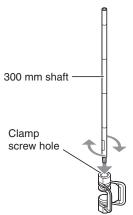
2 Check that the 300 mm shaft is not loose, and then turn the threaded portion of the crankshaft clockwise and tightly fit it into the screw hole of the 300 mm shaft. At this time, lightly tighten the knurled nut until it is at the root position of the threaded portion. Do not open the lantern hanger arm when turning the crankshaft as doing so is dangerous.
