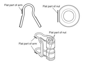
Rotate the bolt counterclockwise and remove it from the nut. Attach the removed bolt to the opposite end of the nut.
