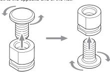
Attach the nut and bolt to the arm by implementing the removal procedure in reverse. Align the flat part of the nut and bolt with the flat part of the arm so that the upper and lower rubber pad surfaces are facing the inside (top plate side). The rubber pads have a non-slip function. Make sure that the rubber pads firmly come in contact with the top plate of the table so that the product will not come off the table.
