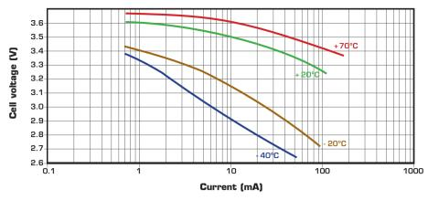
Typical discharge profiles at + 20°C
