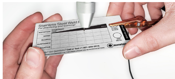
Figure 4.2 Attach the alligator clip to the welding plate. With proper eye protection, hold the welding plate with both hands and lightly touch the electrode to the welding plate. When the electrode contacts the welding plate, the welder will release energy and create a weld.
