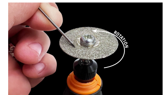
Figure 7.2. A sharp electrode tip improves arc initiation and results in a better overall weld.
