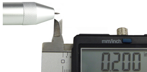
Figure 2.3. Electrodes should protrude past the stylus hull 1/8 to 1/4 inch (3.175 to 6.35mm).
