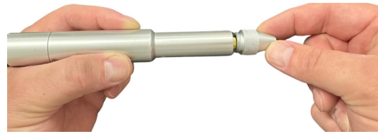
Figure 2.1. To install the electrode, first remove the Stylus Shaft (A) from the Stylus Hull (E) by pulling them apart.
