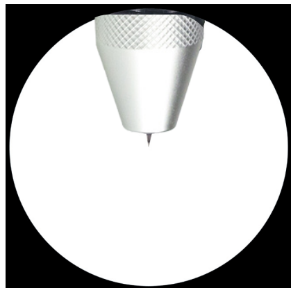
Figure 16.3. Only a small portion of the electrode should extrude from the holder.
