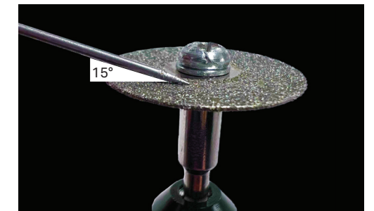
Figure 7.3. Use a rotary tool to sharpen the electrode.
