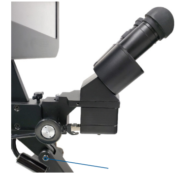
Figure 15.1. Turn this knob to adjust microscope focus. You'll find one knob on each side of the microscope arm.
