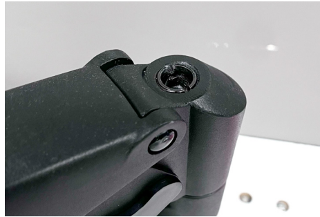
Figure 14.1. Adjust the tension of the Microscope Arm Assembly for more loose or more tight movement.
