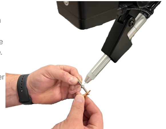
Figure 17.1. Rest your hands on the table and position the workpiece close to, but not touching the electrode. Then look through the microscope.
