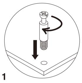
Screw the cam bolt into panel.
