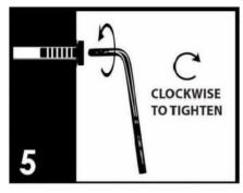
Make sure all parts are properly aligned, then use the appropriate bolts or screws. Do not use power tools and do not overtighten.
