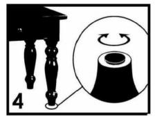
Some furniture comes with height adjusetment knobs underneath each leg. To lower or to raise each leg, volume tool to completely tighten the need to turn clockwise or counterclockwise, respectively.
