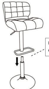
Place the footrest w/handle (#2) onto the gas lift cylinder (#4).
