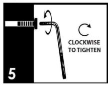
Make sure all parts are properly aligned, then use the appropriate hand tool to completely tighten the bolts or screws. Do not use power tools and do not overtighten.
