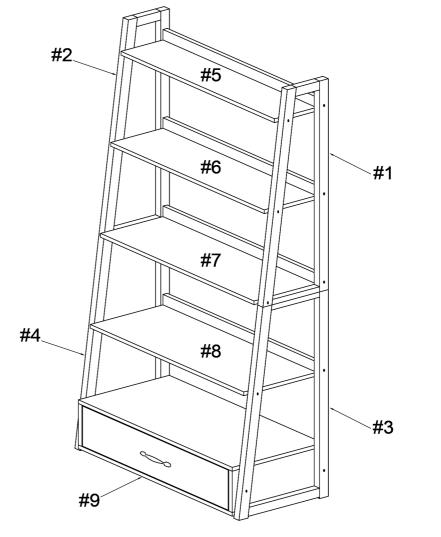
1) Align lower right and left frames (#3,4) to the shelf (#8) and smoking box (#9). Secure frames (#3,4) to shelf (#8) by using bolts (#B) with barrel nuts (#C).
