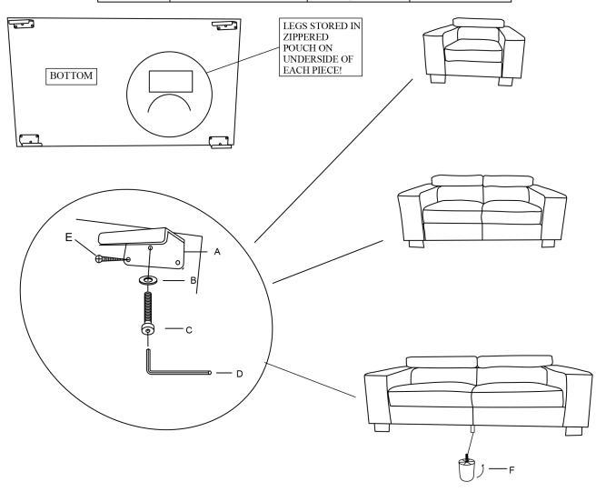
SCREW THE LEGS WITH WASHERS(B) AND ALLEN BOLTS(C) FIRST, THEN SCREW THE WOODEN SCREWS(E) INTO THREADED RECEPTACLES AT THE TWO SIDS OF THE LEG.
