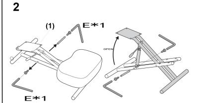
Detach bolts with pin from the footrest (#1), then lift/open the footrest (#1) till the cylinder is aligned to the holes. Secure by using the bolts with pin that was detached.
