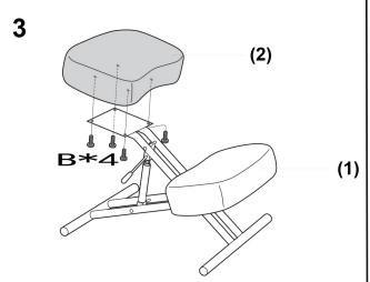
Align cushion (#2) to the footrest (#1), then secure by using bolts (#B).
