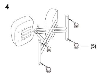
Align and attach the wheels (#5) to the bottom of the footrest frame.
