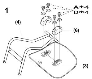
Align support (#4) to backrest (#3), then caps (#6) on top. Secure with bolts (#A) with washers (#D).
