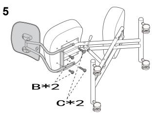
Align backrest to the cushion, then secure by using bolts (#B,C) as shown in the diagram.
