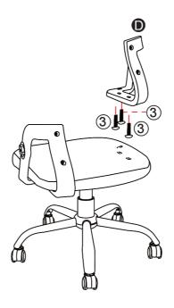
Align chair connector (#D) holes to the bottom of the seat, then secure by using bolts (#3).
