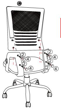
Align chair back (#C) to the holes of the chair connector, then secure by using bolts (#2) with bolt caps (#4).
