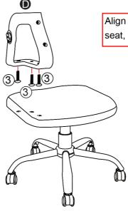
Align chair connector (#D) holes to the bottom of the seat, then secure by using bolts (#3).
