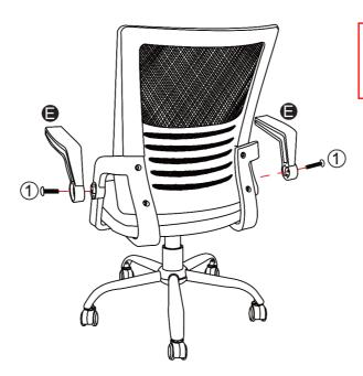
Align armrests (#E) to the chair connectors, then secure by using bolts (#1).
