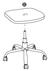
Attach seat (#B) to gas cylinder.
