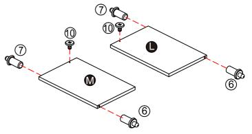
Fixed door pins (#6) are not spring assisted. Only door pins (#7) are spring assisted.
