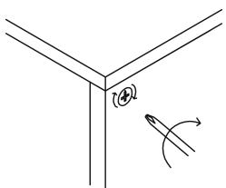
Turn the cam connector with a screwdriver until it will not turn any more with light to moderate force.
