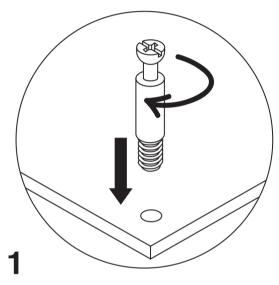
Screw the cam bolt into panel.
