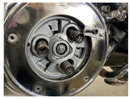
6. Install the 3 tabs shim in the center of the clutch hub. Play with the shim when the VP installed is normal. As the motorcycle is in operation the SDR weighted levers will keep contact on the shim thus the play will be eliminated.
